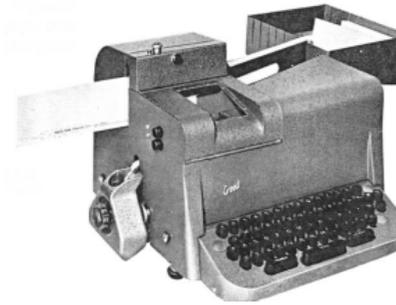
ing Card Punch can either be operated manually from its keyboard or automatically from punched paper tape or edge punched cards, via the appropriate reader equipment.
