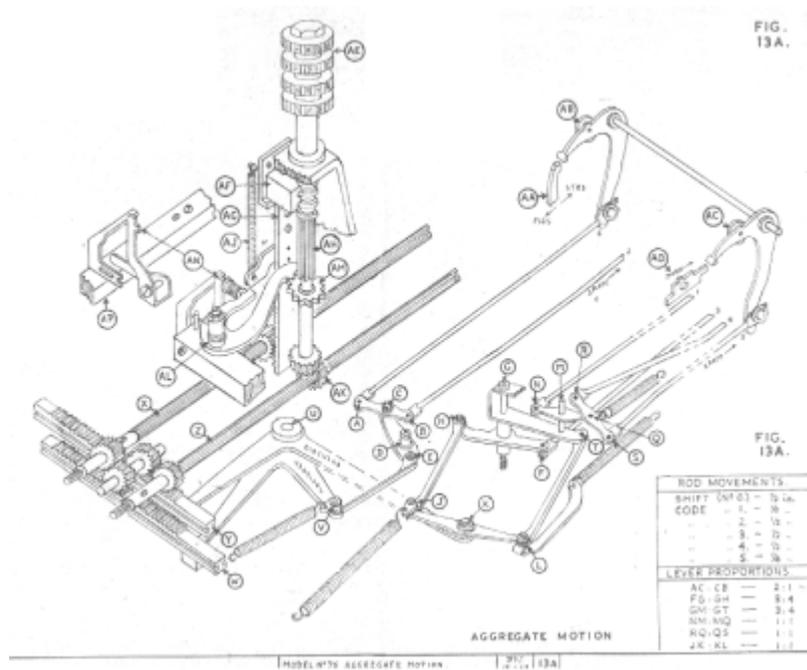
why the Seventy-five is so much smaller than its predecessors. The absence of a bulky carriage moving back and forth allows a saving of something like 7 1/2" in the width of the printer. The stationary platen also eliminates the problems encountered when the paper must follow the to and fro movement of the carriage, and allows the use of page winders for the take-up of printed copy.
